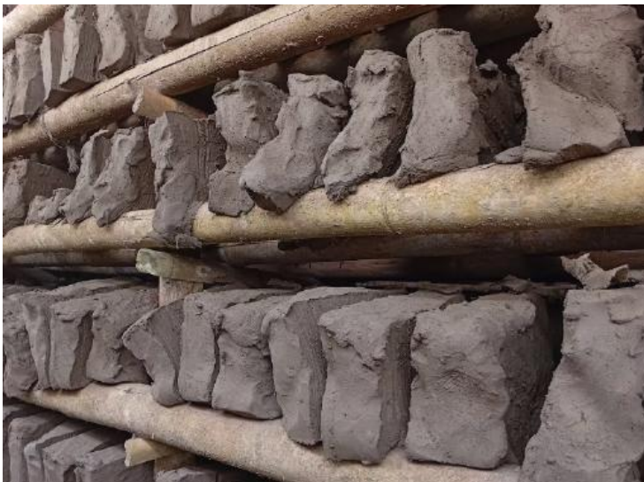
Picture Part of Process Making Roof Tiles
